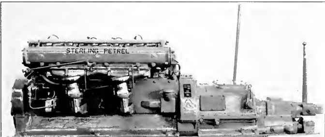
Starboard and port views of the new Sterling Petrel reduction gear gasoline engine fitted with idling clutch.
